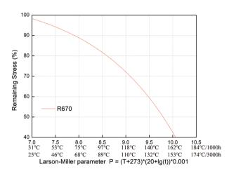
P=Larson Miller parameter T=temperature(<sup>°</sup>C) t=time(h) Example: P=10 is equivalent to 162 <sup>°</sup>C/1000h
